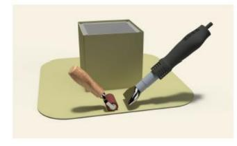
Step 10: Drop down the TPO boot over the roof curb.
